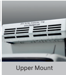
Condensing unit Eutectic cold van HD45 ~ HD170 Operated by 3 phase electric power 380V or 220V with 50Hz or 60Hz. * The condenser Takes the high-temperature, high-pressure gas from the compressor and condenses it into liquid from by cooling it with external air. Note: Standard
